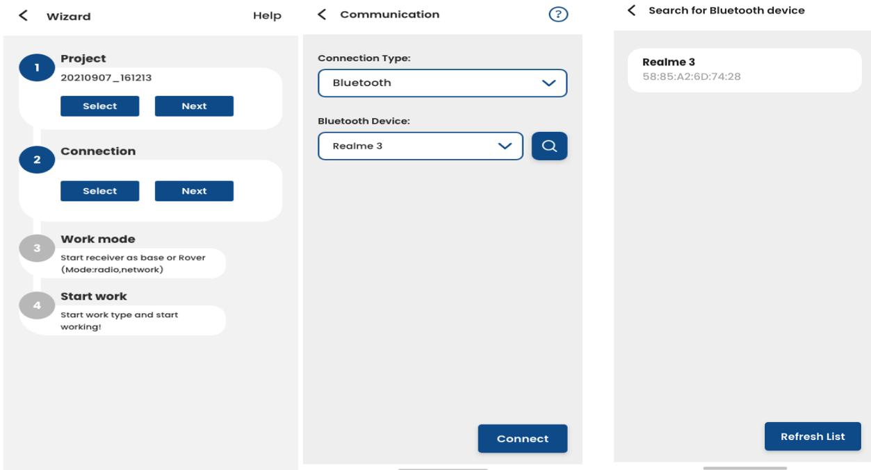
**3. Work mode:** Click select to go into Quick Setup interface to start your receiver as Base/Rover. If you start your receiver as Rover, then you can start work directly of Topo survey or stakeout.
